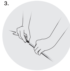
3. Use the plug & play Power Kit to assemble the lamp
