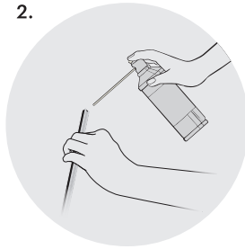
2. Carefully remove any aluminum burrs, dust, debris or shavings
